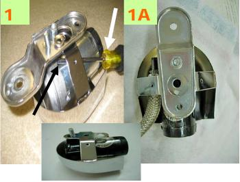
There are 3 holes in cover, USE THE <u>TOP</u>HOLE. Place flat side of regular screwdriver under head of 3/4" bolt for support while fastening 5/16"lock washer and 5/16" nut (PICTURE 1) Once compressor is installed, it will NOT be visible. Completed assembly (PICTURE 1A).
