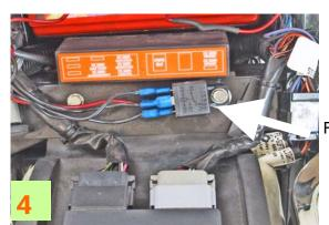
Final step is to mount and wire relay under seat (PICTURE #4).
